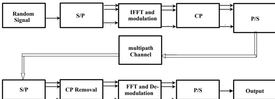
Fig. 4 Block diagram of OFDM transmitter and receiver
