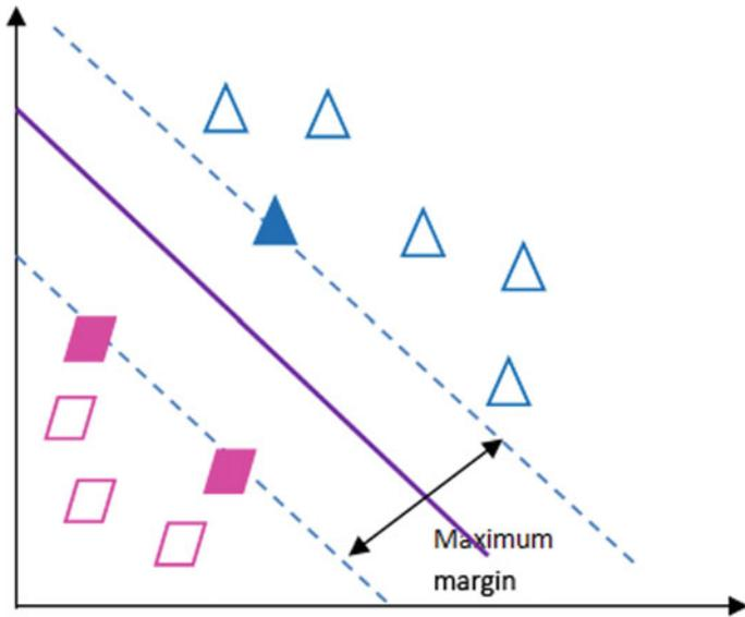
Fig. 5 Support vector machine classification
