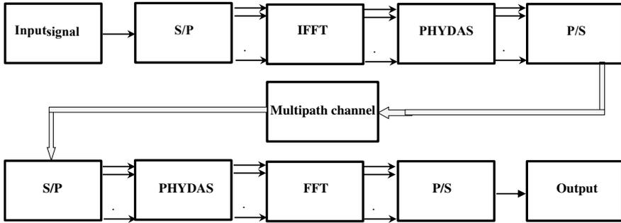
**Fig. 5** FBMC block diagram
