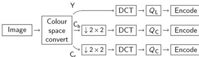
Fig. 5 Functional steps of JPEG image compression
