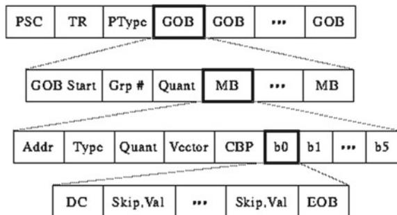
The group of blocks (GOB) component of the bitstream indicates the separation of the picture into  $11 \times 3$  macroblock regions. The group number (Grp #) indicates whole groups that should be skipped and the group quantization value (GQuant) indicates the single quantization value for the whole group.
