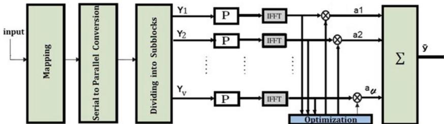
Fig. 8 Proposed modified PTS technique
